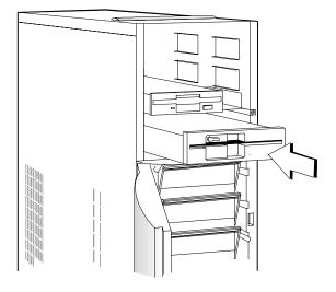
Figure 3-12. Inserting the Drive into the Drive Bay
